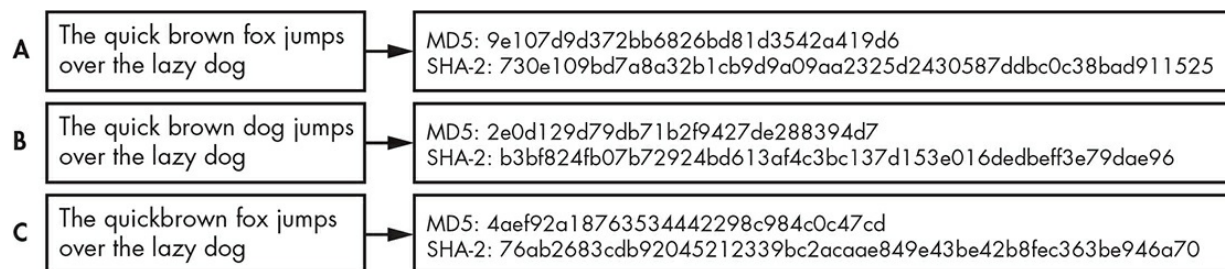
Figure 5-7: A hash function generates a unique value for every message, no matter how similar the messages are.
