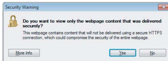
Figure 7-9: Browsers present a warning when a page accessed over HTTPS contains items accessed over HTTP.
